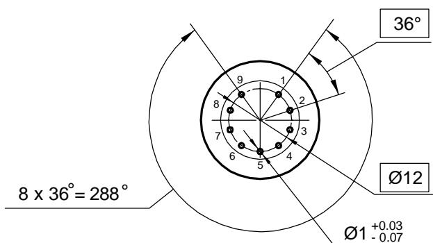
Electrode -to - lead connection diagram
