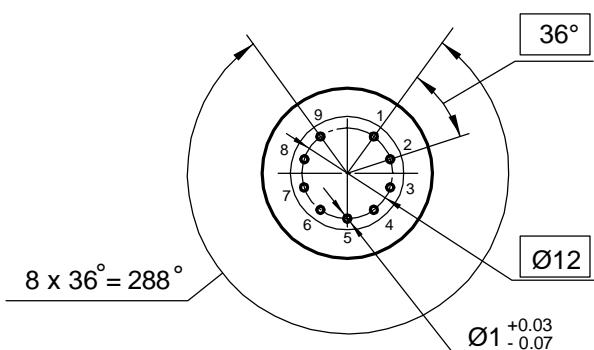
Electrode -to - lead connection diagram
